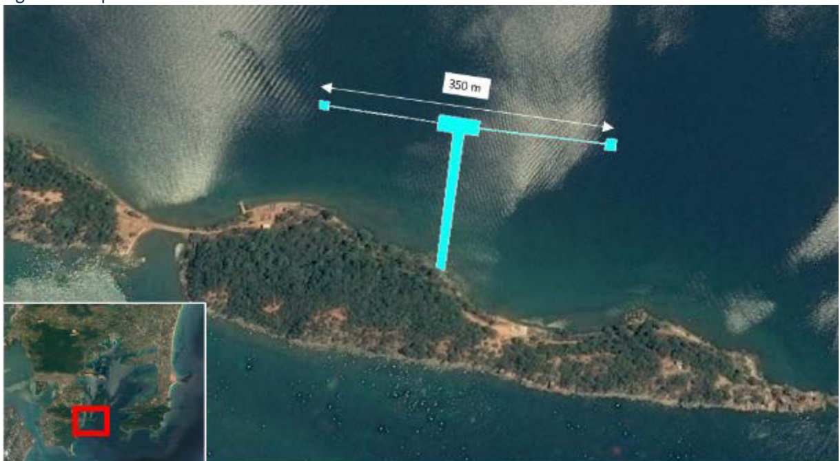
Figure 9-8: Options Accommodation LNG Hub Terminal
