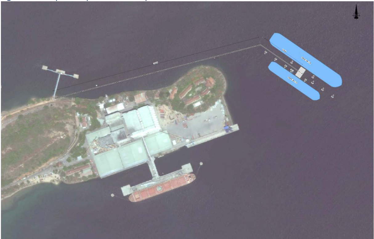
Figure 12-3: Proposed Lay-out of New Jetty
