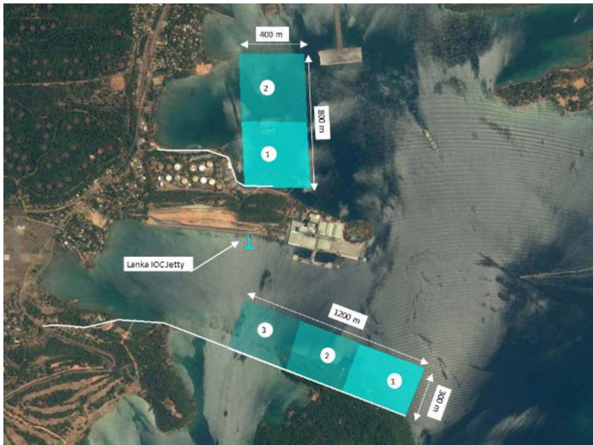
Figure 9-12: Two Options Accommodation Container Terminal
