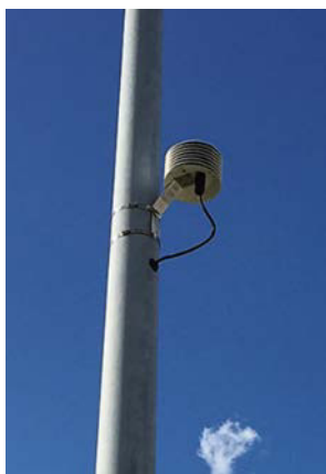
eNose mounted onto a lightpole.
